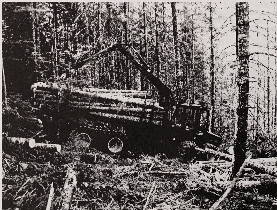
Forwarder loading logs on Camas East Density Management Thinning
