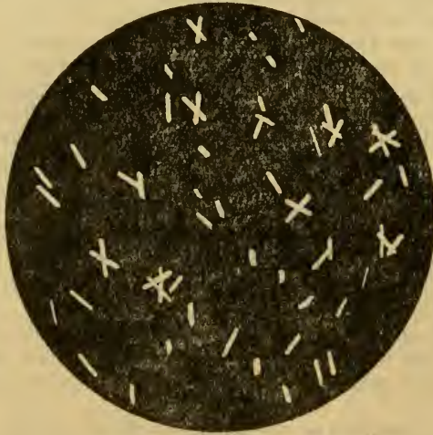
FIG. 1.—Crystals and fragments of guanin from pearl essence derived from shad. Magnification approximately 100 diameters
