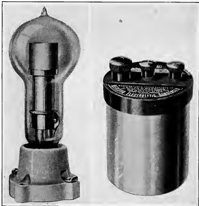
FIG. 20.—Cold cathode rectifier and electrolytic condenser.
