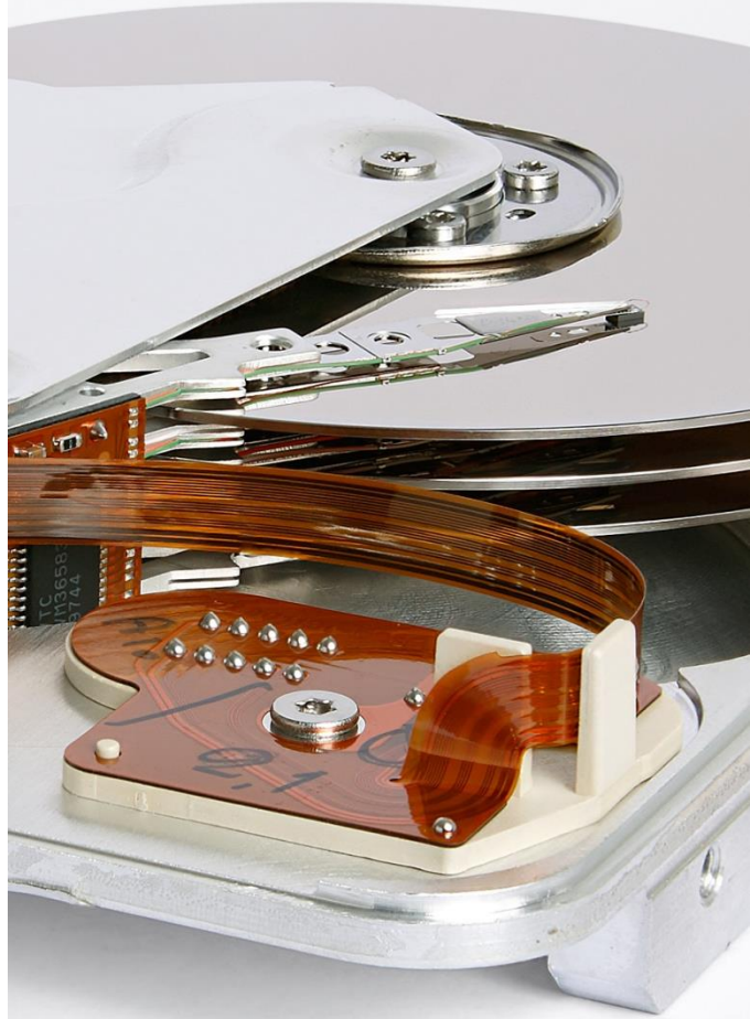
Eric Gaba, Seagate ST33232A hard disk inner view, CC-BY-SA 3.0
