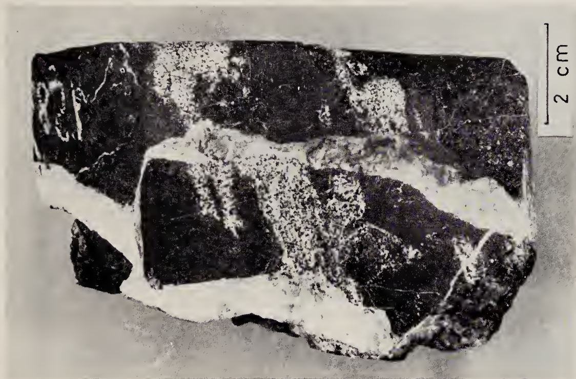
FIG. 2.—Rodngite veins (white) transecting and offsetting schlieren-banded (spotted and streaky) chromite with serpentine minerals) and massive chromite ore (black) from the Mooney Trig Mine, North Mooney Ridge.
