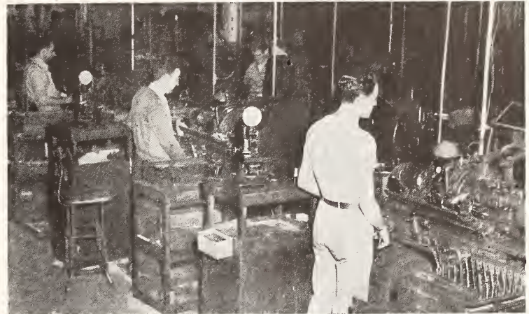
Visual control of operations—a bank of cylindrical grinders with instruments to check tolerances of 20/1000th of an inch.
