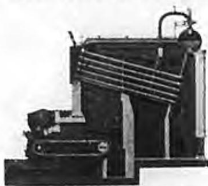
CT Type Water Tube Boiler
