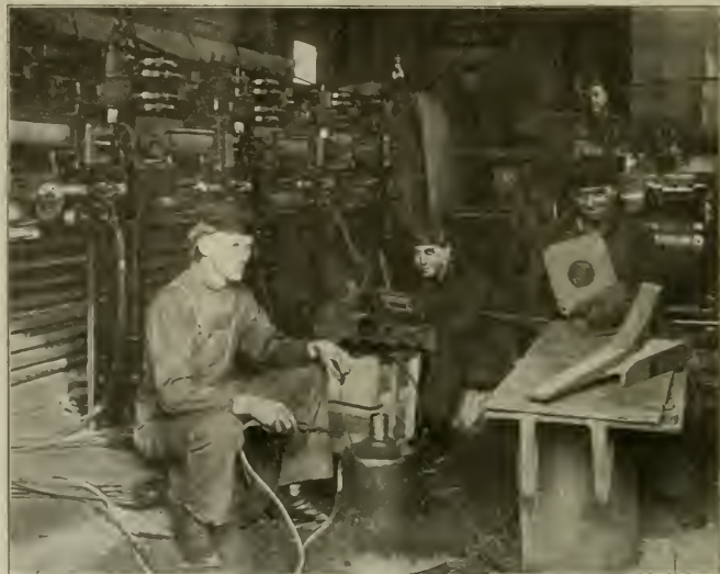
VARIETY OF OPERATIONS AT ONE AND THE SAME TIME WITHOUT INTERFERING WITH EACH OTHER. FOUR OPERATORS WELDING FOUR DIFFERENT METALS, EACH WITH A DIFFERENT AMPERAGE FROM A SINGLE GENERATOR.
