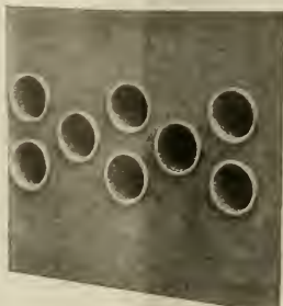
SECTION OF LOCOMOTIVE FLUE SHEET WITH TUBES WELDED BY METALLIC ELECTRODE.
