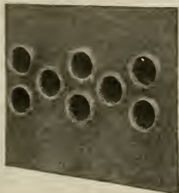
SECTION OF LOCOMOTIVE FLUE SHEET WITH TUBES IN PLACE READY FOR WELDING.
