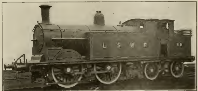
LONDON AND SOUTH WESTERN ENGINE EQUIPPED WITH STOP SIGNAL APPARATUS
