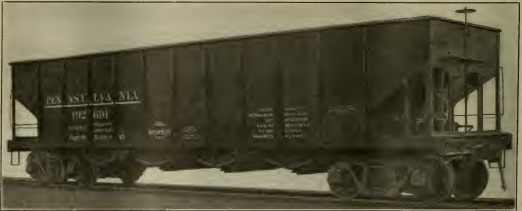
SEVENTY-TON STEEL GONDOLA BUILT FOR THE P. R. R. BY THE CAMBRIA STEEL COMPANY
