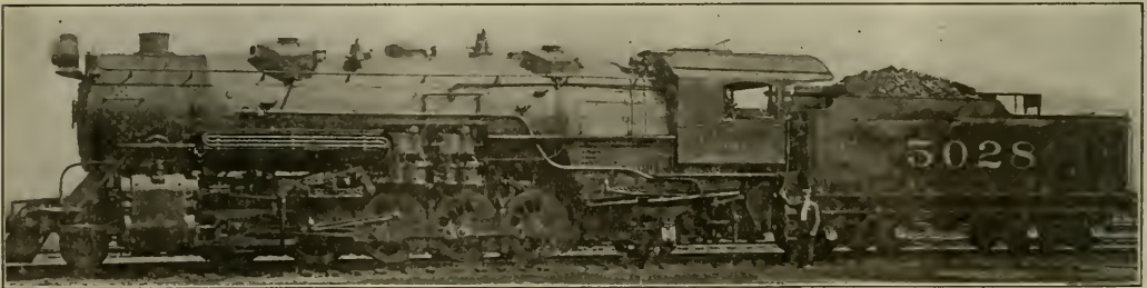
2-10-2 ENGINE FOR THE SOUTHERN, EQUIPPED WITH THE HANNA STOKER.
