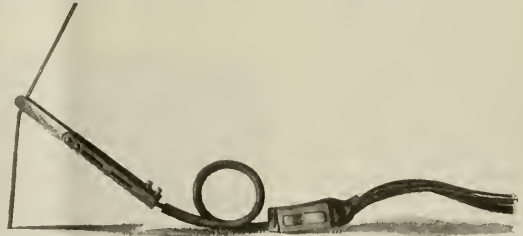
WELDING TOOL OR ELECTRODE HOLDER WITH DISTANT CONTROL SWITCH.
