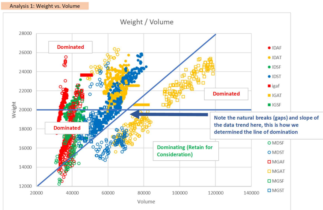
Figure 17: Set Based Design analysis comparing variants of a medium-surface combatant [65]
