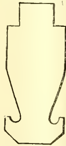
FIG. 63.—MESSRS. FOSTER AND PEARSON'S IMPROVED GLAZING-BAR.
