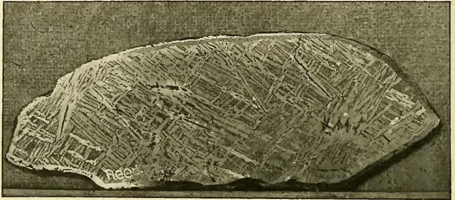
FIG. 2.—Section showing Widmanstätten figures. Three-fifths actual size.
