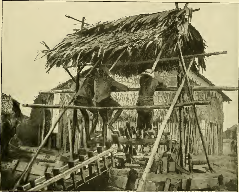
FIG. 7.—Pumping water by human treadmill, near Lahat, Perak, Malay peninsula.
