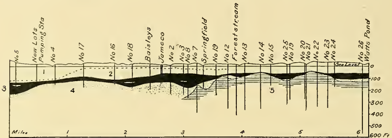
FIG. 5.—Section along the line ab of Fig. 4, showing portions of (1) Wisconsin; (2) Manhasset; (3) Sankaty; (4) Jameco; (5) Cretaceous beds, and east side of old valley. Numbers refer to the Brooklyn water-works test wells.
