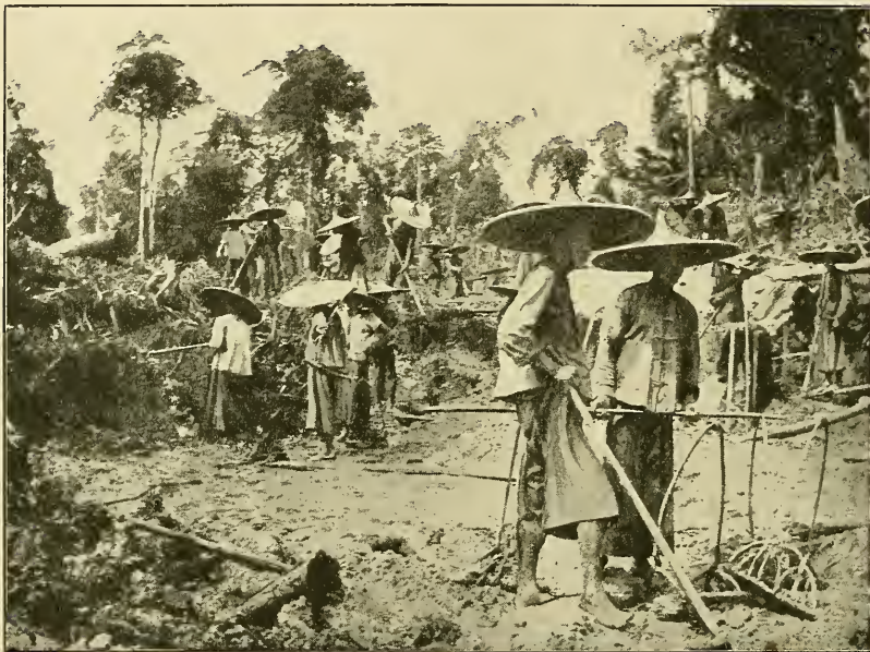
FIG. 3.—Stripping new tin ground south of Campar, Perak, Malay peninsula.
