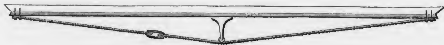
Fig. 2. Rafter, with Wire rope Supporter.
