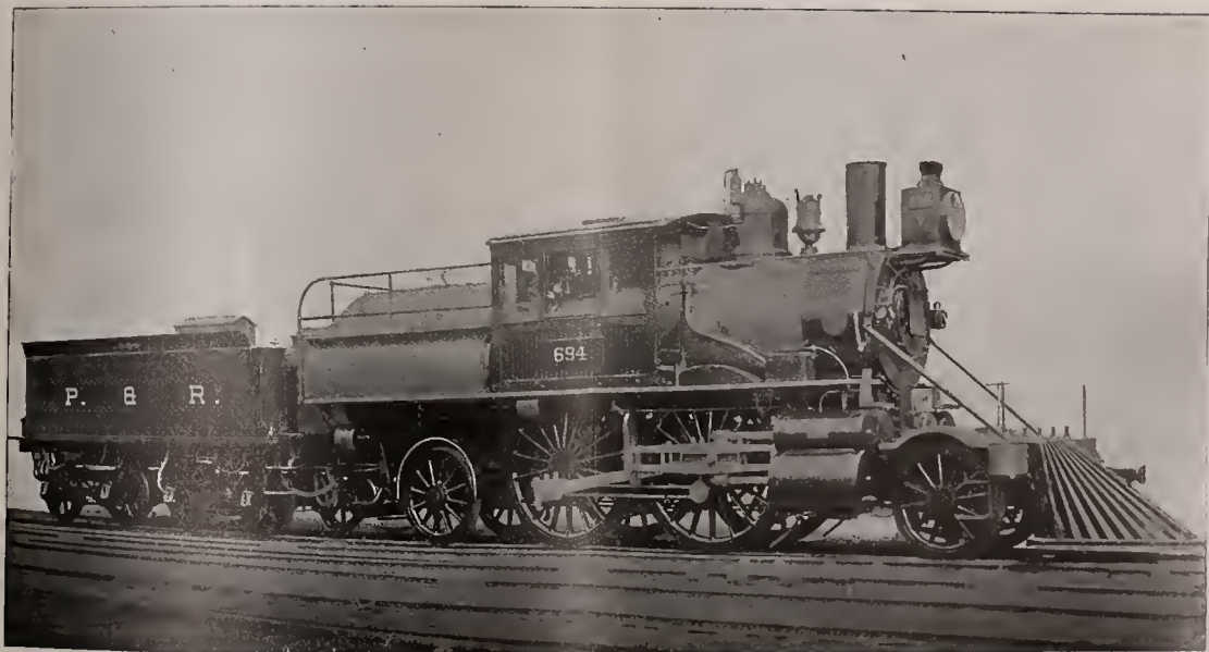
PLATE VII.—Compound Express Passenger Engine, No. 694, Philadelphia & Reading Railroad. Built by Baldwin Locomotive Works.
