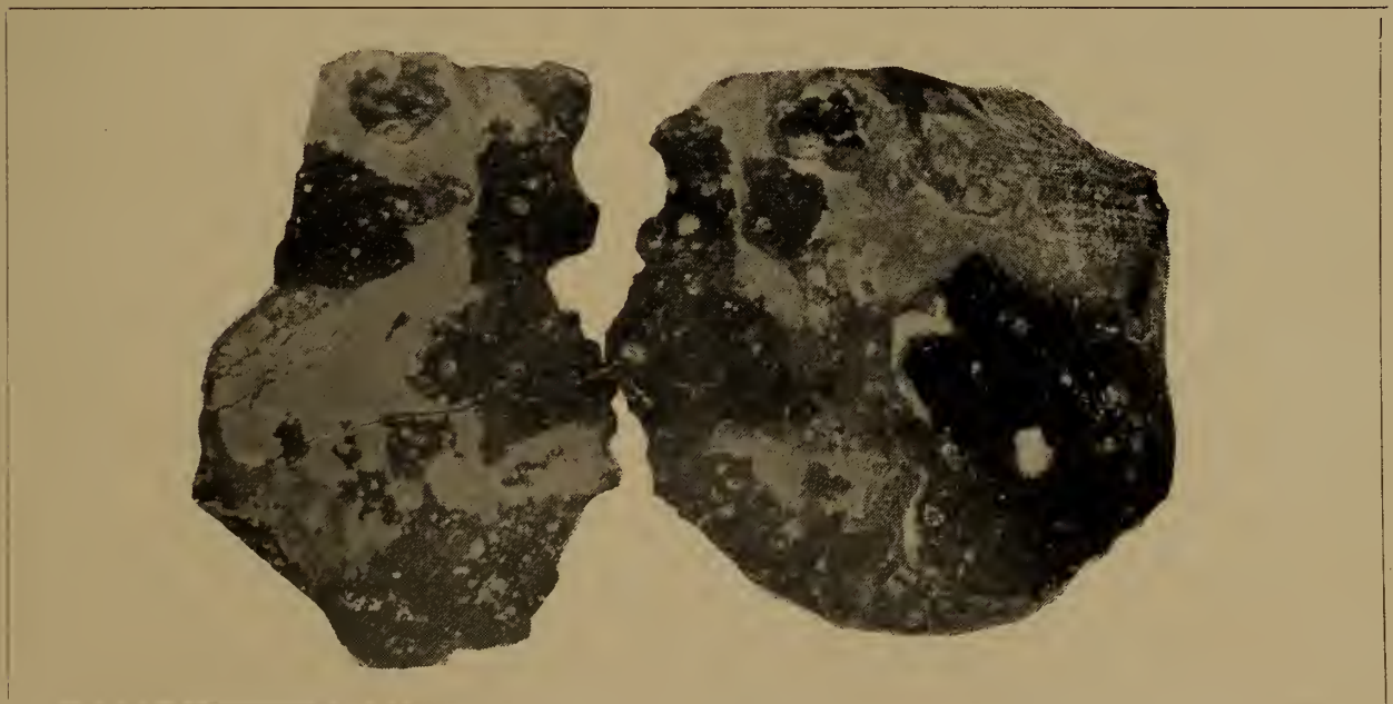
FIGURE 2.—POLISHED PIECES SHOWING MIXTURE OF TRAP AND MUD
