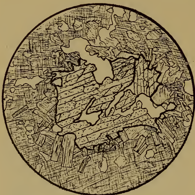
FIGURE 3.— Augite Phenocryst with Rim of Biotite, from Black Rock Butte.
