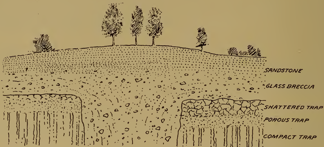
FIGURE 2.—Generalized Section of Overflow of Glass Breccia through Trap north of Meriden.
