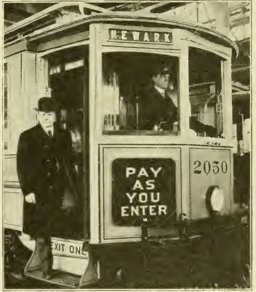
Pay-As-You-Enter Cars for Public Service Railway—View of Front Platform.
