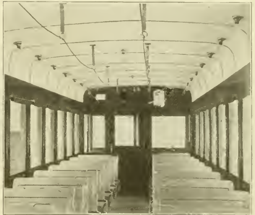
Long Single-Truck Cars Without Monitors—Interior of Car No. 14, Showing Arrangement of Lamps, Register and Ventilator.
