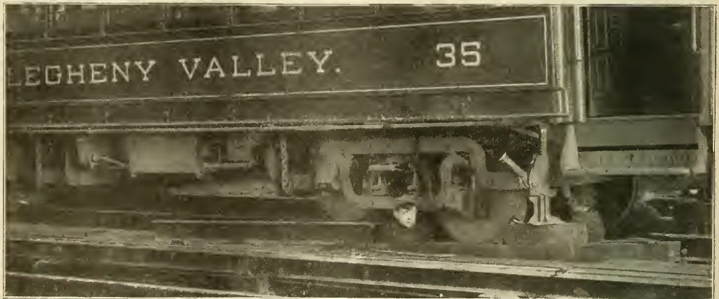
Allegheny Shop Practice—Method of Supporting Body and Truck When Changing Wheels on Interurban Equipment.
