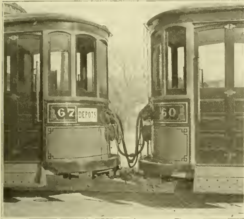
Multiple Car Operation in St. Joseph, Mo.—Air and Coupler Attachments Between Two Motor Cars.
