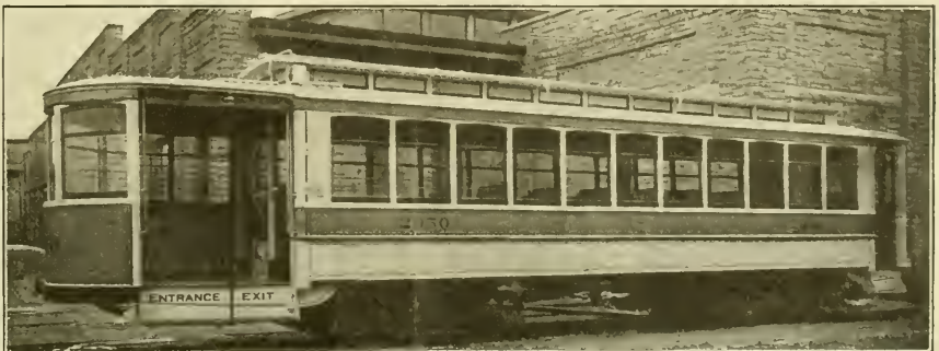
Type "Pay-as-you-enter" Cars. 200 Built for The Public Service Railway Company, New Jersey
