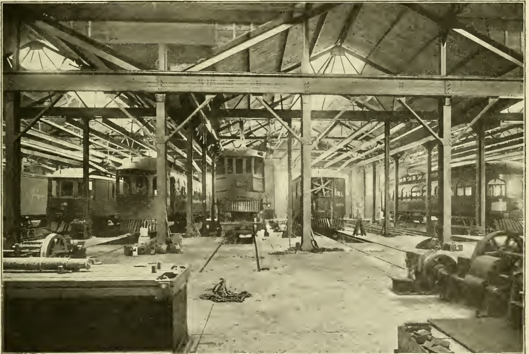
Anderson Shops Indiana Union Traction Company—Car Repair Shops, Showing Car Body Being Raised by Two Electric Hoists.
