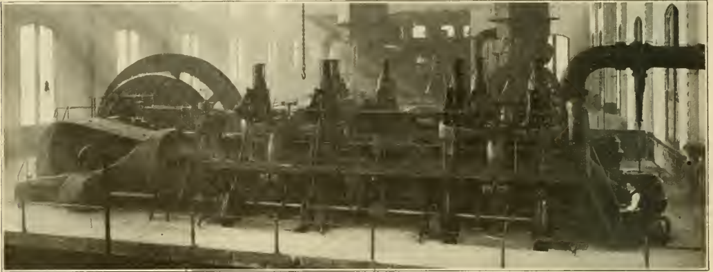
Westinghouse Horizontal Double-Acting Gas Engine—Engine at the Bessemer Plant of the Carnegie Steel Company.
