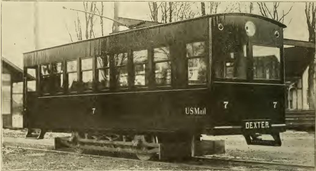
Long Single-Truck Cars Without Monitors—Car No. 7. Twenty-eight Feet 6 Inches Long, Without Monitor, 10-Foot Wheel Base.
