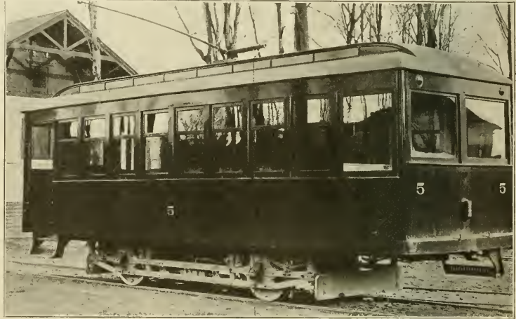
Long Single-Truck Cars Without Monitors—Car No. 5. Low Monitor, Square Ends and 10-Foot Wheel Base.
