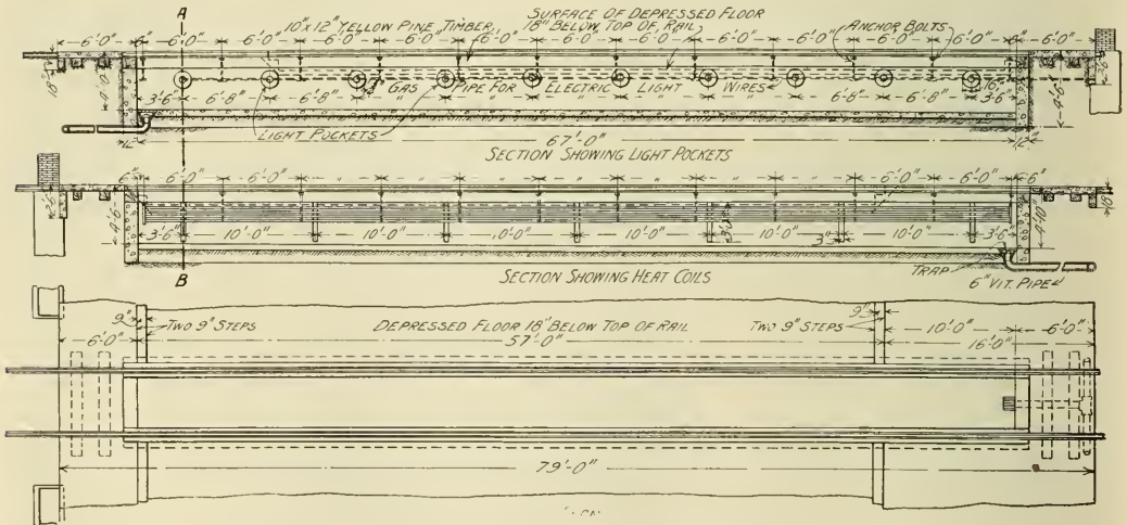
Anderson Shops Indiana Union Traction Company—Details of Repair Pits.
