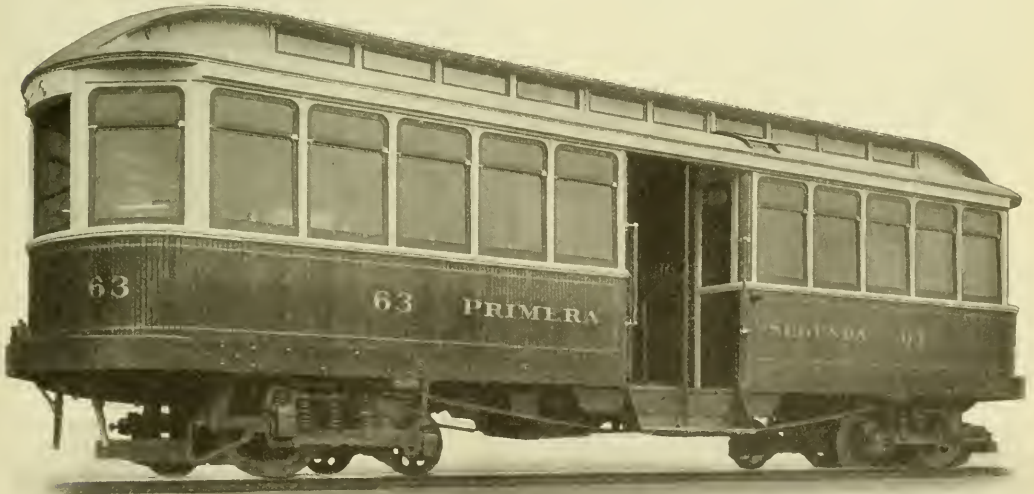
Pay-As-You-Enter Cars for Monterey, Mex.—Exterior View, Showing Center Side Entrance.
