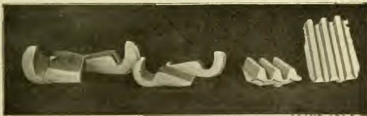
Baltimore Shops—Plaster of Paris Impressions from Wheels and Gears.
