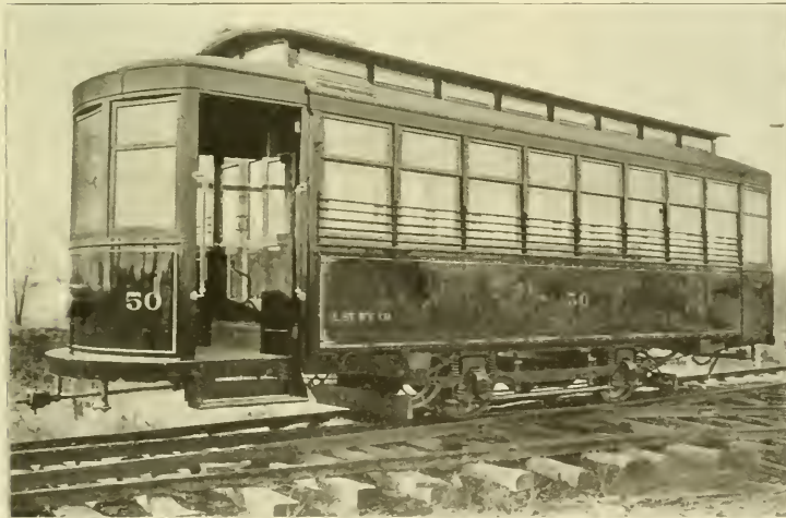
Semi-Steel Car—Amarillo Street Railway.
