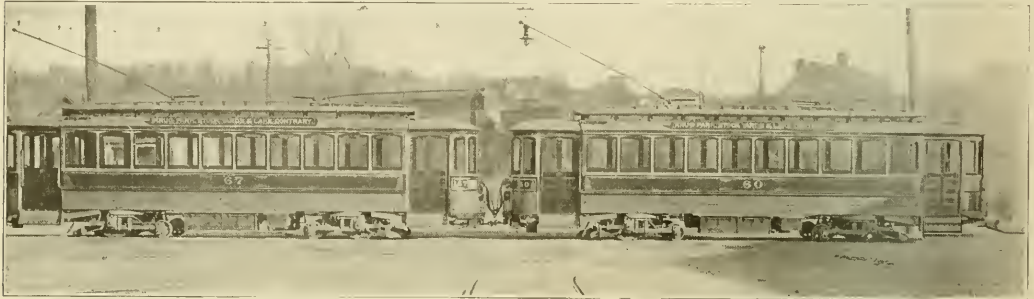
Multiple Car Operation in St. Joseph, Mo.—Two Motor Cars Coupled for Multiple Operation.
