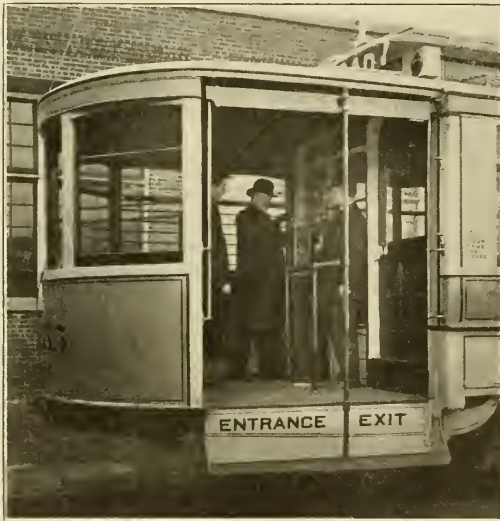
Pay-As-You-Enter Car in Newark—View of Rear Platform, Showing Position of Fare Box.
