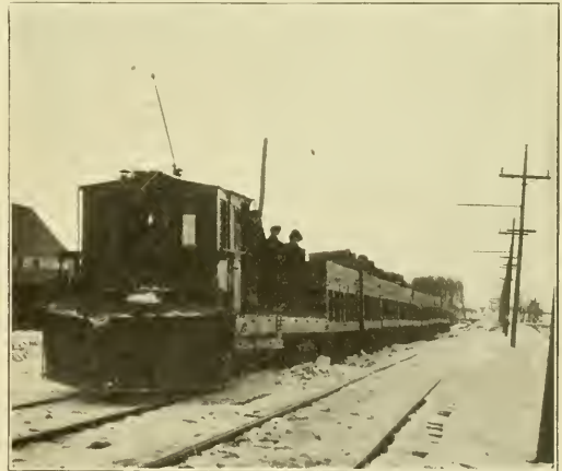
Chicago & Southern—Combination Work Car, Snow Plow and Ballast Spreader.
