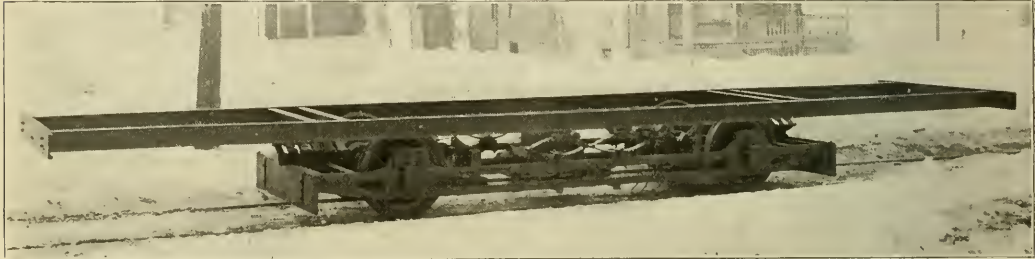
Long Single-Truck Cars Without Monitors—Side View of Steel Underframe and Running Gear for 35-Foot Single-Truck Car. Wheel Base, 12 Feet.
