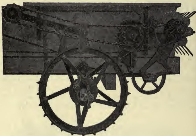
FIG. 148—A CHAIN DRIVE TO THE BEATER. NOTE THE METHOD OF REVERSING THE MOTION
