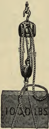
FIG. 5—A TACKLE. A FORCE MAY BE MULTIPLIED MANY TIMES BY A TACKLE OF THIS KIND
