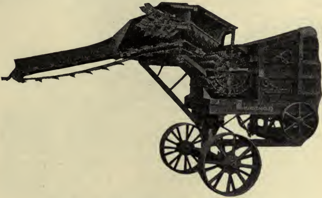
FIG. 162—A SECTIONAL VIEW OF A SELF-FEEDER
