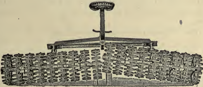
FIG. 61—A FLEXIBLE ROLLER AND CLOD CRUSHER OF SPECIAL DESIGN
