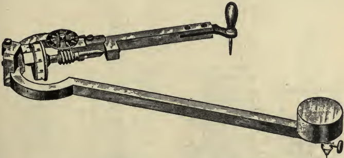
FIG. 13—THE PLANIMETER USED TO FIND THE AVERAGE DRAFT FROM DYNAMOMETER RECORDS. THERE ARE SEVERAL TYPES OF THIS INSTRUMENT
