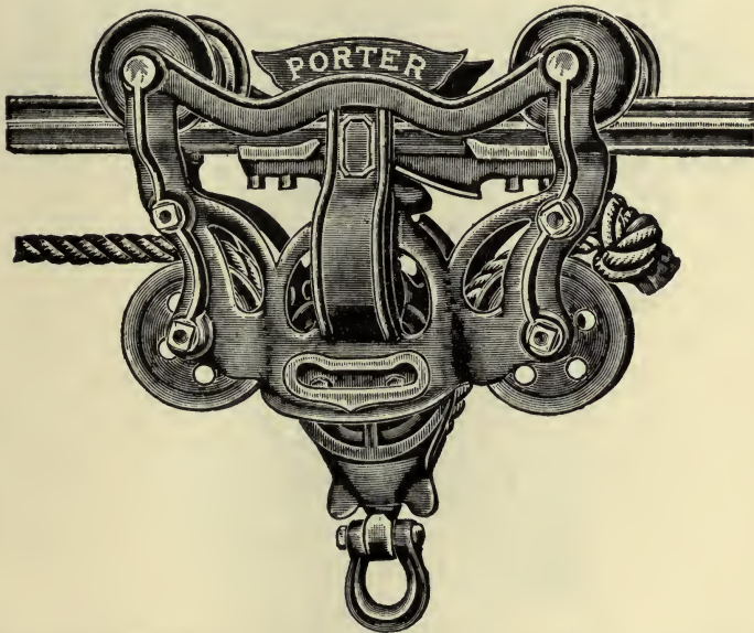
FIG. 140—A TWO-WAY FORK HAY CARRIER. TO WORK IN THE OPPOSITE DIRECTION, THE ROPE IS SIMPLY PULLED THROUGH UNTIL THE KNOT ON THE OPPOSITE END IS STOPPED BY THE CARRIER
