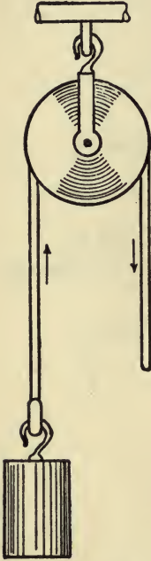
FIG. 4—SIMPLE PULLEY, WHICH ONLY CHANGES THE DIRECTION OF A FORCE
