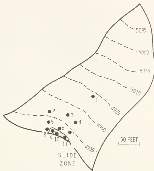
Figure 13. — Location of piezometers and limits of slide zone, Watershed No. 4, Pine Creek study area.
