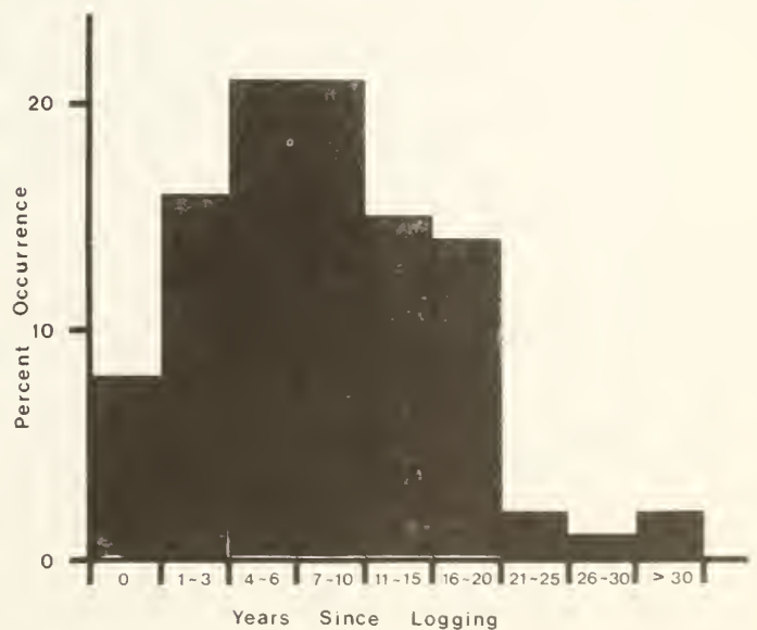
Figure 7. — Landslide occurrence by years since logging, western and central Northern Rocky Mountain province (from Megahan and others 1978).
