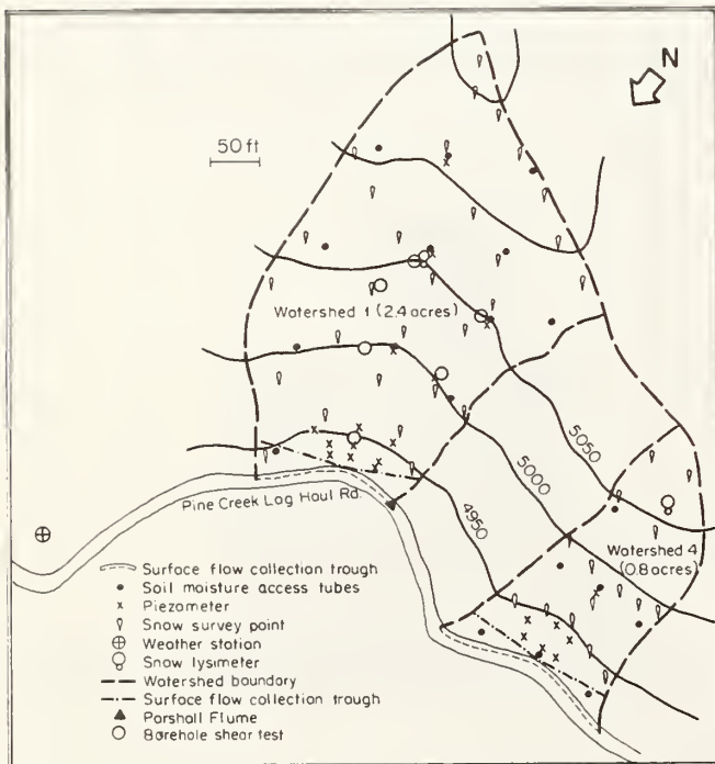
Figure 8. — Pine Creek study area showing location of instrument and data collection stations in the watersheds.
