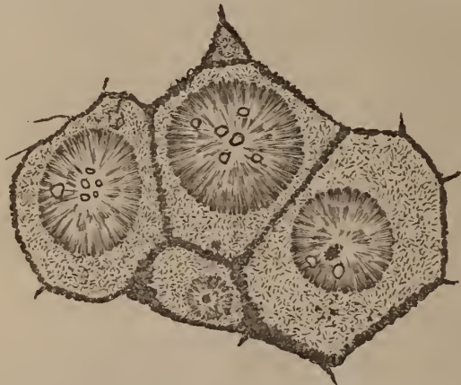
FIG. 3.—Spherulitic Felsite. Diagrammatic sketch from microscope. The radial structure in the spherulites is rather exaggerated; the exterior granulated part with both prisms shows 'felsitic' structure, sometimes with slight radial tendency, the polygons are defined by opaque clotted (ferruginous?) dust.
