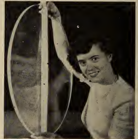
Polaroid's new 22½-inch lens for sharpening up theater Tv images.
