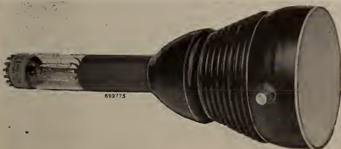
The 7NP4 projection Kinescope used with the RCA PT-100 theater Tv system.
