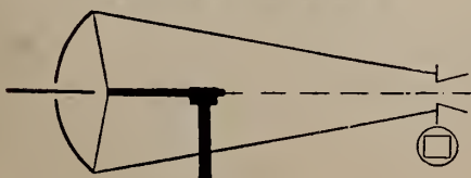
FIG. 1. Representation of an arclamp optical system using a concave mirror.
