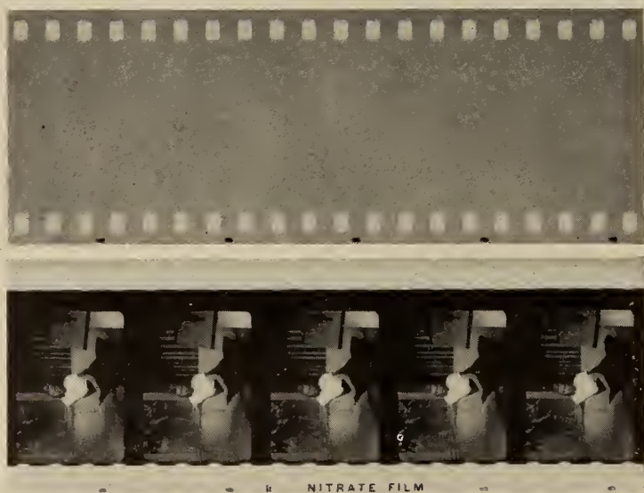
FIG. 5. The visible frame-line mark on raw and processed nitrate film manufactured by Canadian Kodak.
