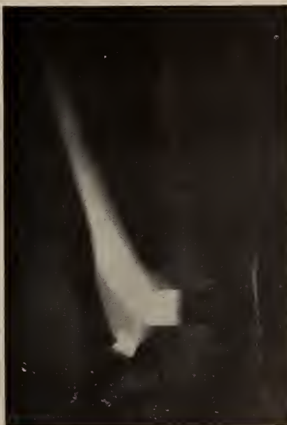
FIG. 5 (a). The arc burning with no air supplied from jet, the characteristic long tail-flame reaching toward the optical system.
