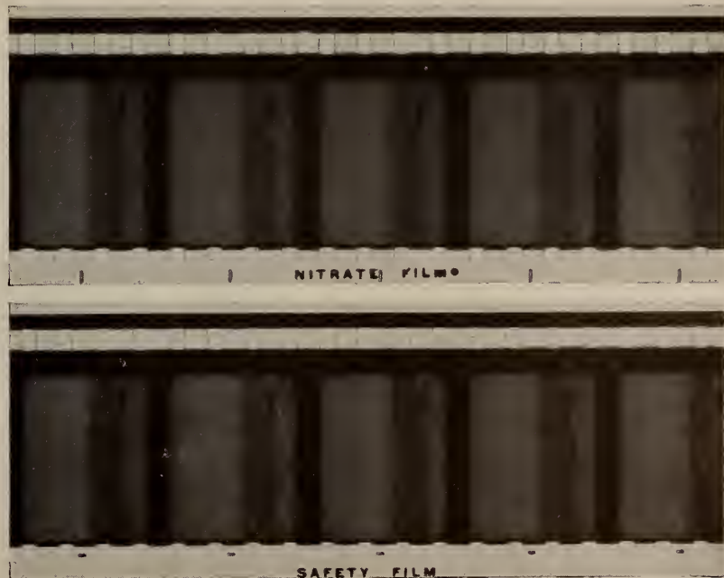
FIG. 4. The new Eastman visible frame-line mark on processed safety film compared with nitrate.
