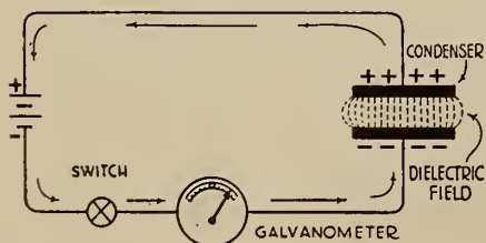
FIG. 1. Charging a condenser.
