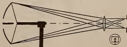
FIG. 2. Optical system utilizing concave mirror and intermediate-image formation.
