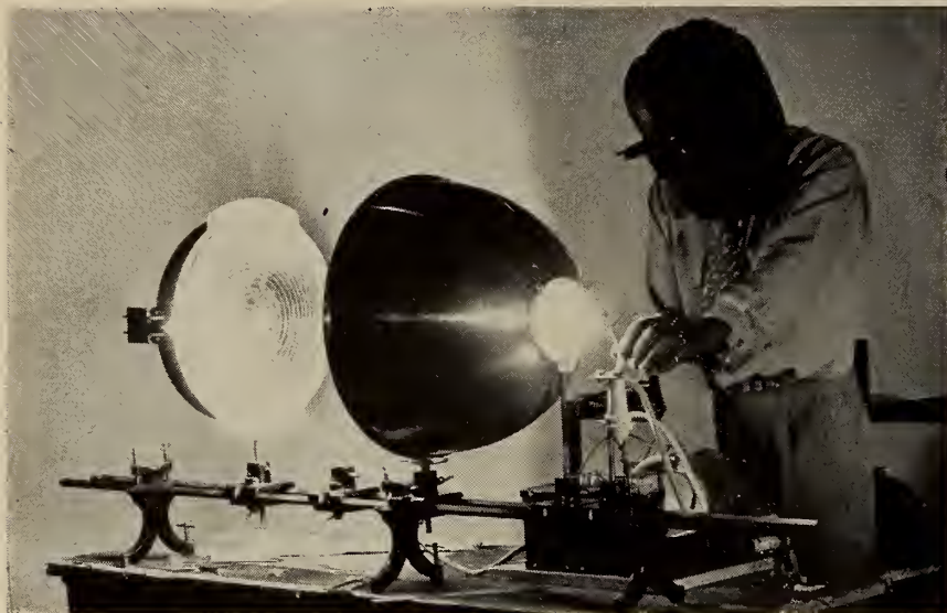
FIG. 1. Mercury-cadmium lamp under test.
