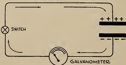
FIG. 2. Discharging a condenser.
