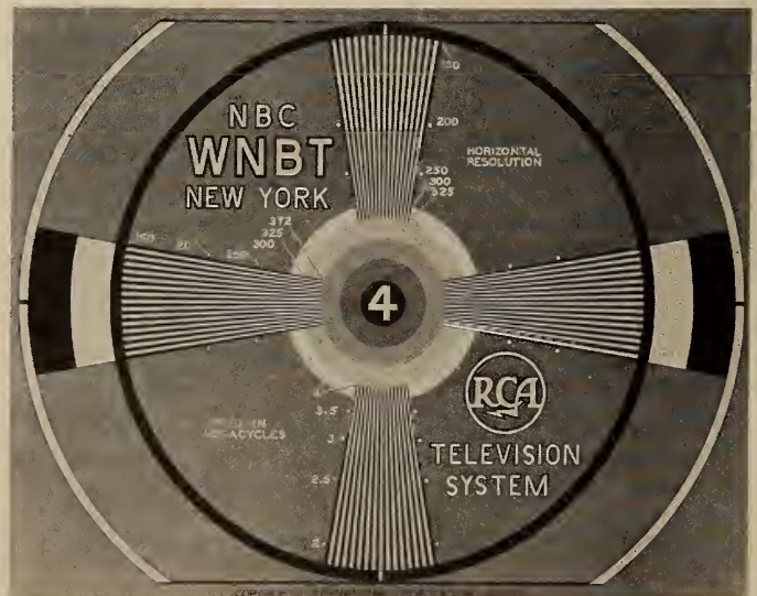
FIGURE 1 A typical Tv test pattern put on the air by the broadcast station for checking band width of the signal, picture resolution, and correct adjustment of controls.
