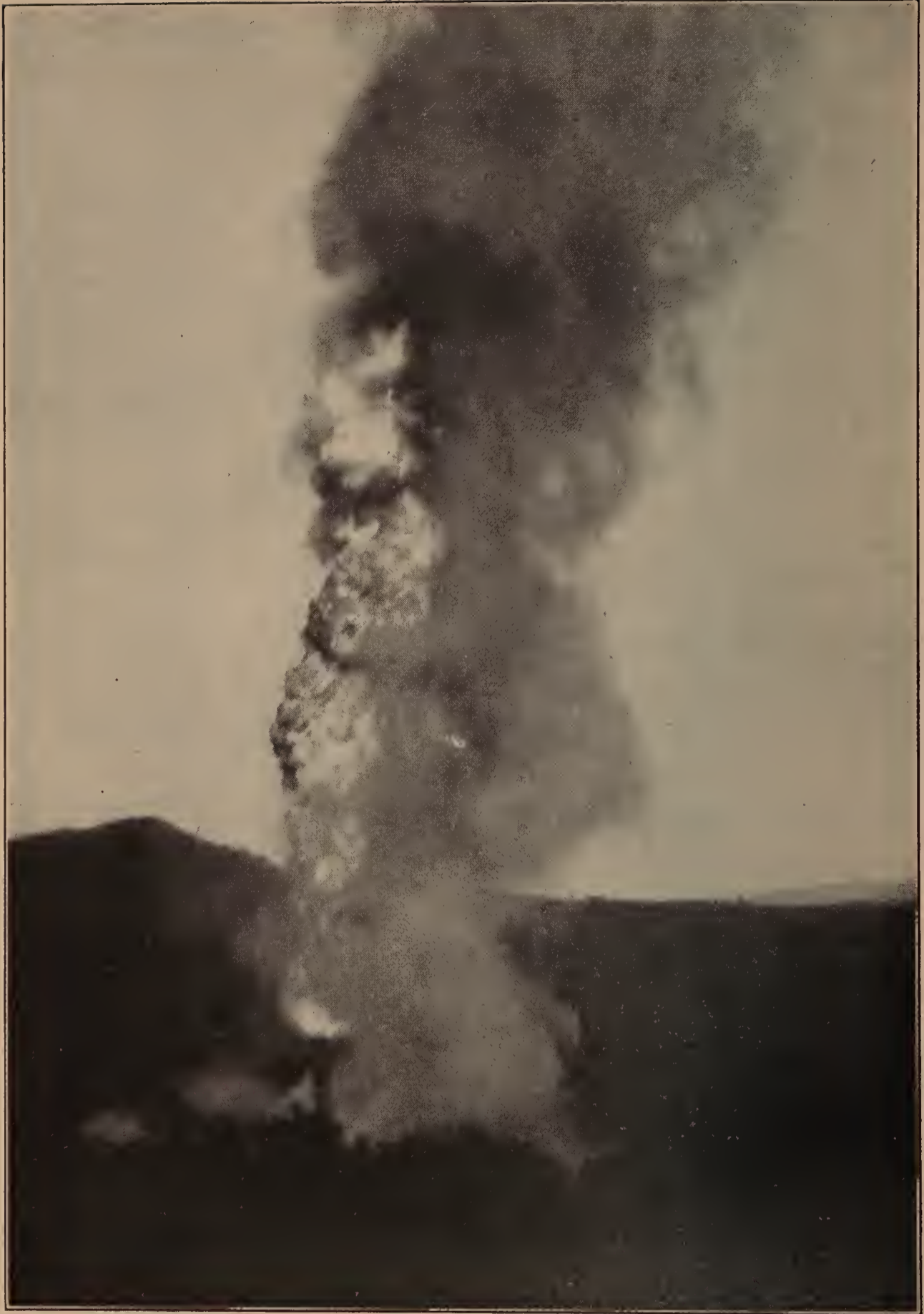
Sometimes when a big well comes in the pressure blows the drilling tools up against a steel block in the derrick striking a spark that ignites the oil and making a great blaze which it may take weeks to extinguish.
