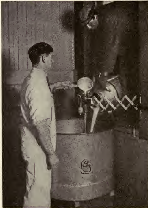
Fig. 81.—A simple aid to sediment testing. This convenient method of fastening the sediment tester by means of a telephone bracket is a handy time saver. (Bull. 241, July, 1914, Univ. of Wis. Agri. Exp. Sta.)
