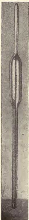
Fig. 45.—A pipet holding 17.6 c.c. of milk used in the Babcock test. (Circular of Information No. 27, July, 1911, Univ. of Wis. Agr. Exp. Sta.)
