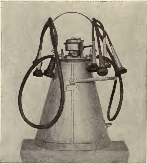
Fig. 124.—Milking machine used in experiments by Lane and Stocking. (Bull. No. 92, B. A. I.)
