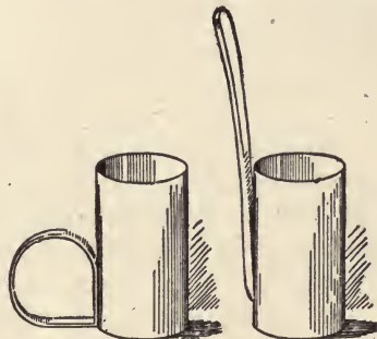
Fig. 237.—Ice-cream samplers. The kind for use with containers having a large diameter. (Benkendorf.)
