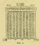
same size wire, carefully tried for carrying the full current of the machine at all speeds. With the fire proof regulator, the motor can therefore be slowed down and left running at any desired speed indefinitely; and the usual caution. "never to leave the box half turned on for fear of overheating and fire," is unnecessary. The capacity of these boxes is stamped upon them also, as it is on all apparatus made by the company.
