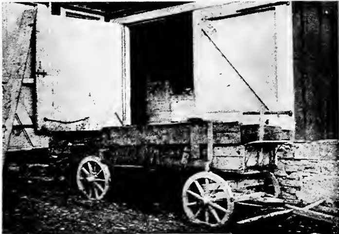
110. MANURE WAGON, WHICH RECEIVES THE MANURE FROM THE STALLS AND FROM WHICH IT IS SPREAD ON THE LAND EACH DAY
