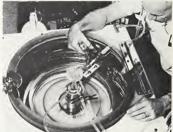
This centrifuge is used to purify specimens of respiratory viruses, such as influenza, parainfluenza, and respiratory syncytial, for various studies including vaccine development.
