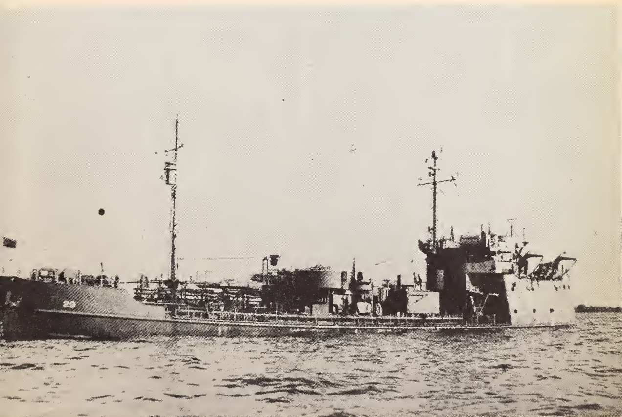
YO Fuel Oil Barge (YO-29 carried Diesel oil) YOG (gasoline) same as YO's
