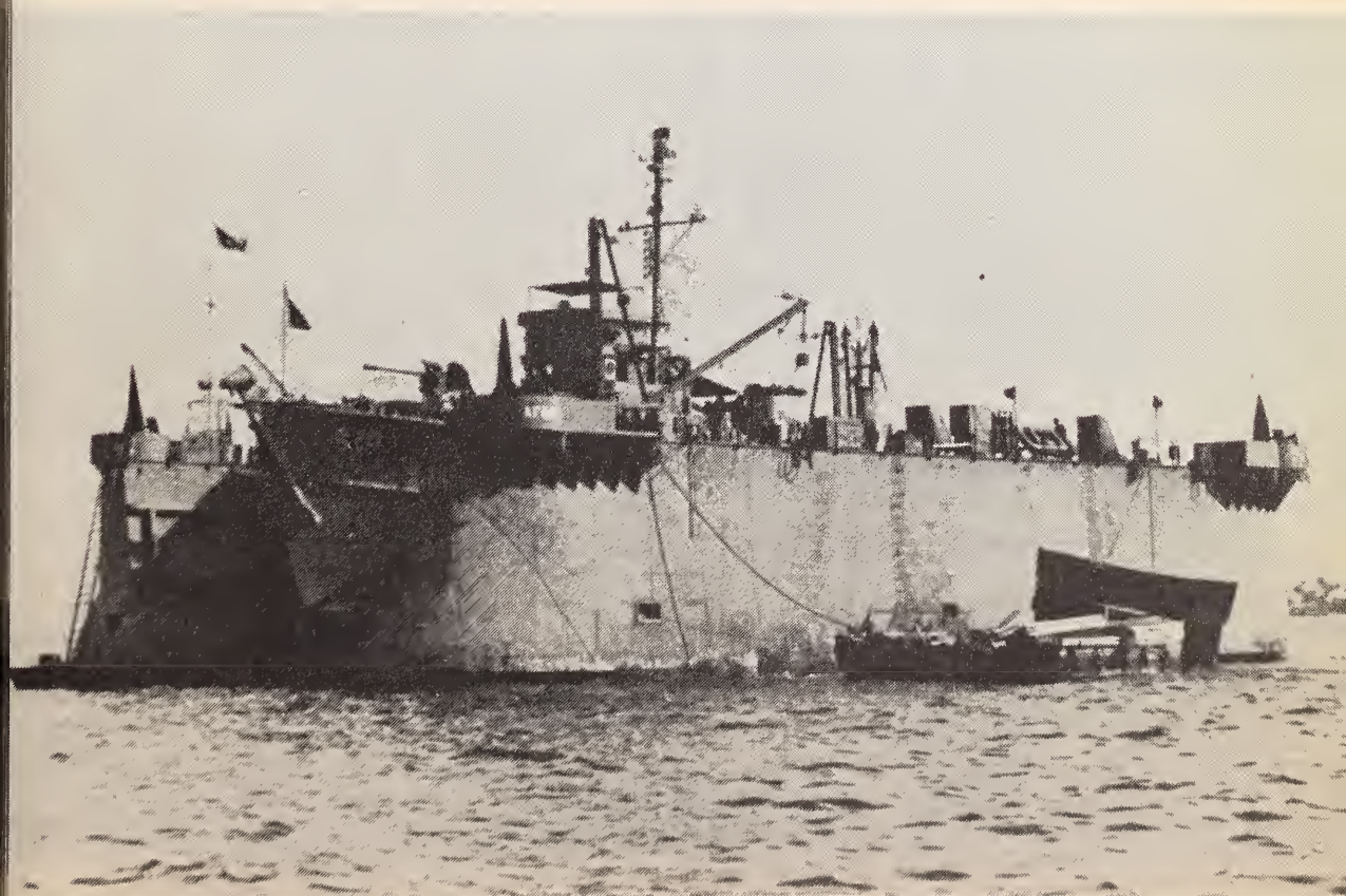
AFD Mobile Floating Drydock (AFD-5) 1000 tons
