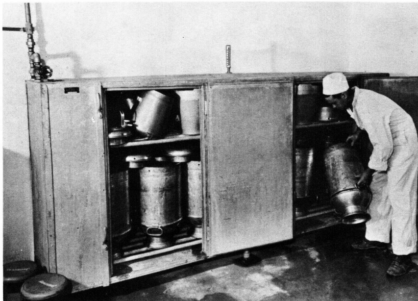
FIGURE 11.—A well-made steam cabinet, showing coils and thermometer.
