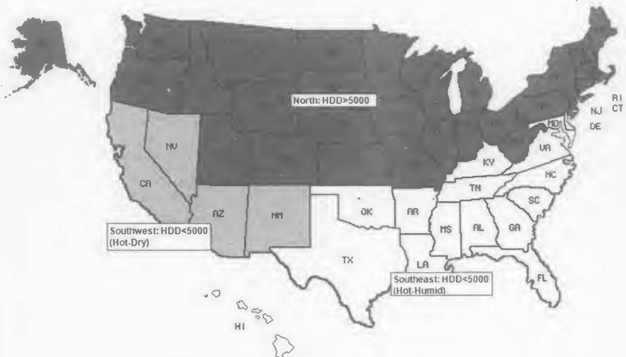
Figure III.3 Map of the Regions for the Analysis of Central Air Conditioners and Heat Pumps
