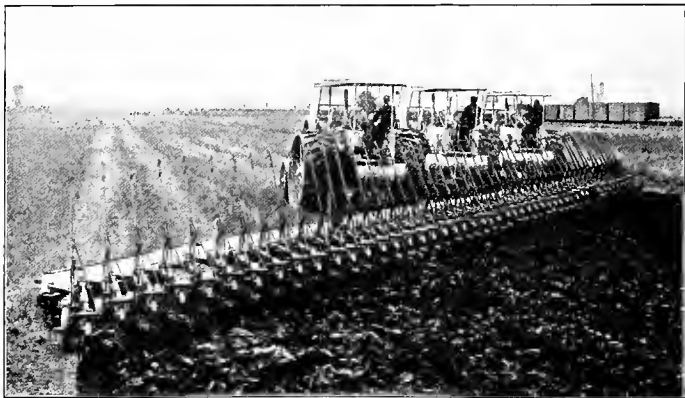
FIG. 5. The "Oil Pull" Gang Plough, which, in a demonstration in 1911, with three engines, did the work of 100 men, 200 horses, and 50 ploughs, ploughing 14 acres an hour at a fuel cost of 6½ cents per acre.
