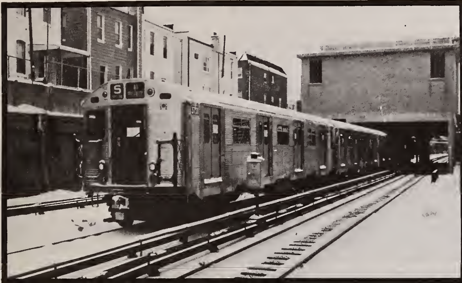
The Garrett energy storage cars underwent testing on New York City Transit Authority lines during the winter of 1975-76.
