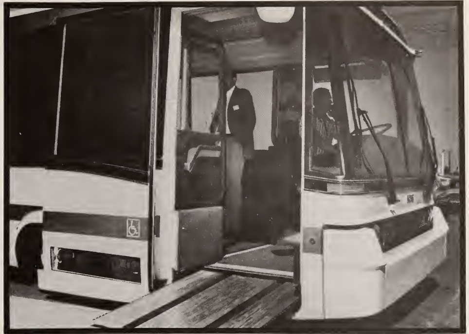
Special wheelchair lift or ramp mechanisms, such as this Transbus feature, are being considered for use as optional original equipment on current design buses.
