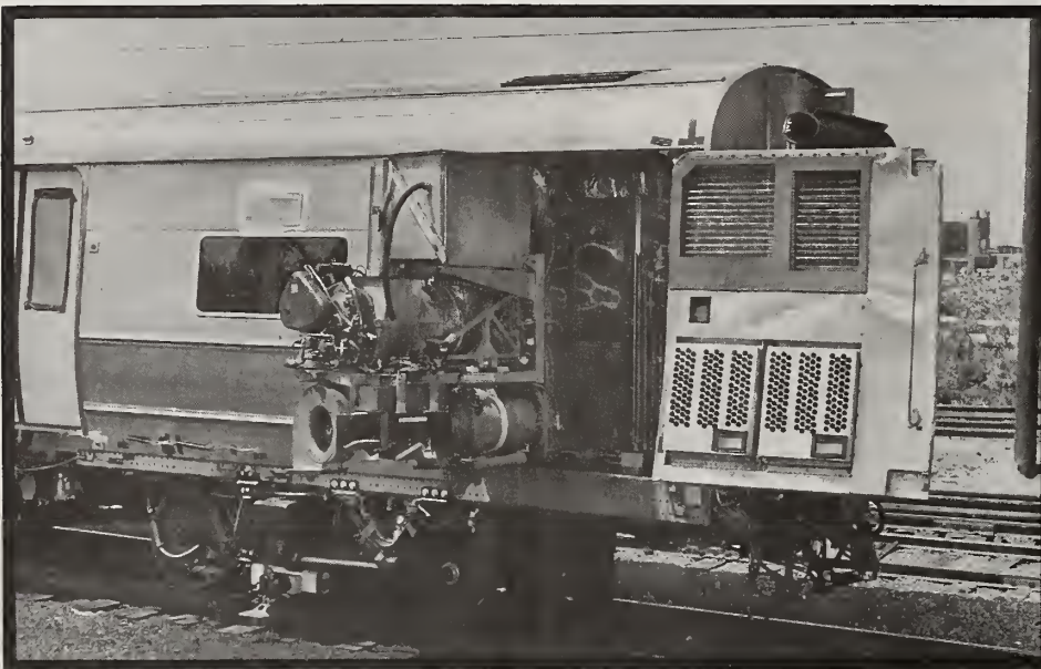
The General Electric Gas Turbine/Electric prototype car is equipped with a slide-out turbine engine for easy maintenance.
