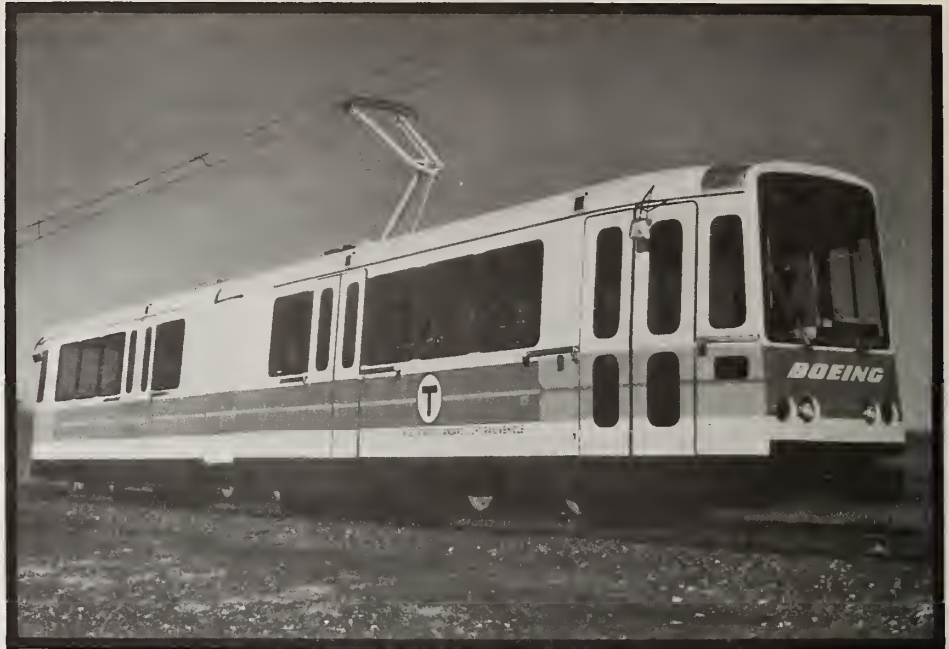
The new Standard Light Rail Vehicle, developed in the United States with UMTA assistance, was one of many programs worldwide studied in a comprehensive light rail transit analysis.
