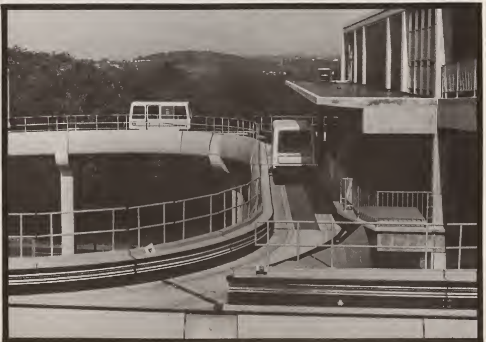
The Morgantown, West Virginia, Personal Rapid Transit system, one of the most innovative systems in the nation, uses rubber-tired small vehicles that run on elevated fixed guideways.
