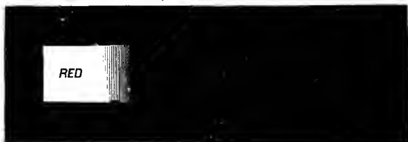
FIG. 15.—Spectrum of Light transmitted through Red Glass.
