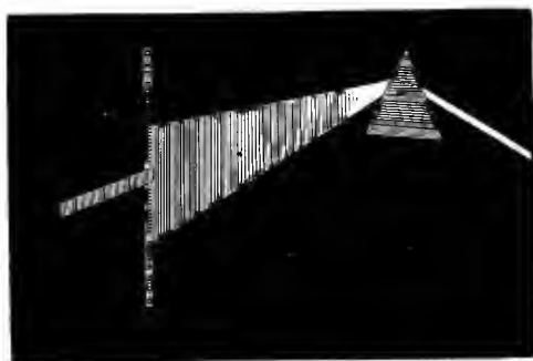
FIG. 2.—Mode of isolating a Single Colour of the Prismatic Spectrum.
