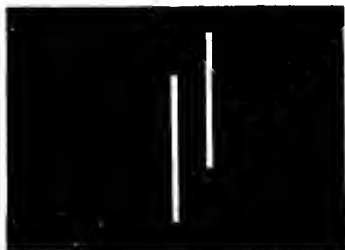
FIG. 41.—Two Slits arranged for mixing Two Spectra.
