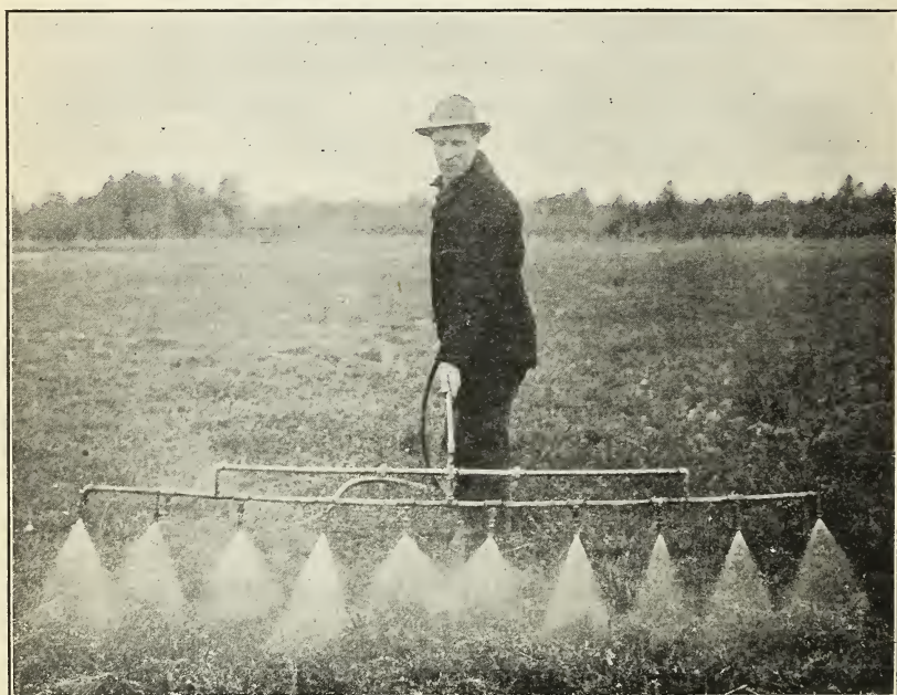
FIG. 15.—A spray boom for holding 10 Vermorel nozzles. Note the unevenness of the spray cone and the necessity of considerable walking and dragging of hose over vines in spraying. Not a good type of outfit to use.
