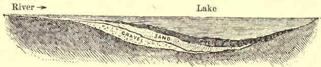
Fig. 1. The order of deposition of river-borne sediments on the floor of a lake after a recent flood. After Lapworth.
