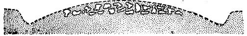
FIG. 3.—Cross section of road, showing lumps of clay placed on a sand subsoil and covered with sand.
