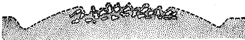
FIG. 4.—Cross section of road, showing displacement of lumps of clay when subjected to travel.
