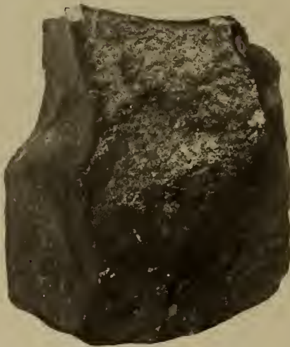
FIG. 5. Primary crust at left. Tertiary crust beginning as a smoky alteration. \times 0.85 diameters.
