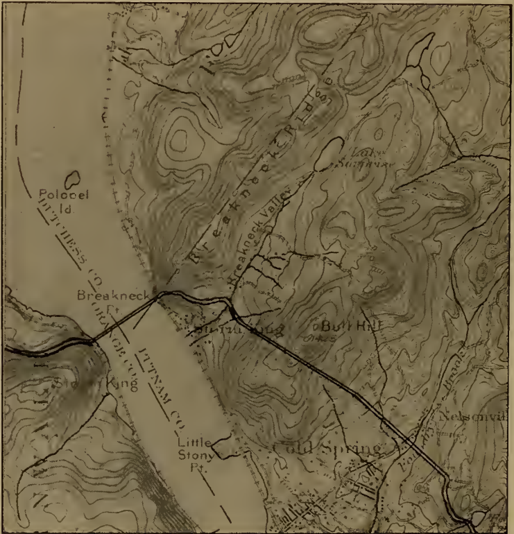
FIG. 3. Topographic map showing the approaches of the aqueduct to the Storm King Crossing. Below and above the 400 contour, there is tunneling.
