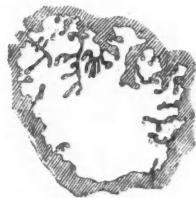
Fig. 26.—Dendrite from a blowhole. Chernoff.
