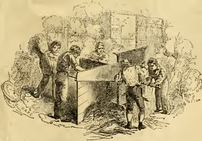
MESSRS. BARRETT, EXALL, AND ANDREWES' (OF READING) HAND THRASHING MACHINE AT WORK.
