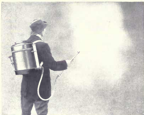
FIG. 169.—A KNAPSACK SPRAYER ("FOUR OAKS PATENT") USEFUL IN SPRAYING BUSH FRUIT, ETC.
