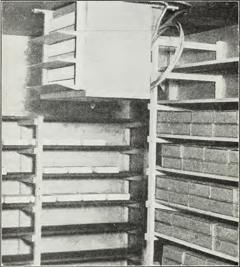
FIGURE 13.—Part of curing room, showing cheeses partly cured before wrapping, and individual cartons each containing a wrapped cheese which ripens 2 to 6 weeks more. Also shows refrigeration unit (of direct-expansion type).
