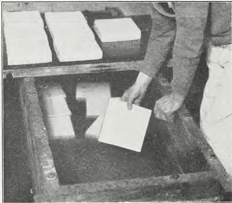
FIGURE 9.—Removing cheese from the brine tank. Tanks may be of cement, brick, tile, or wood construction.
