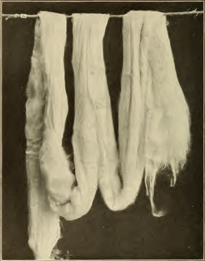
FIG. 18.— Spreader lap of dressed silk ready for preparing in the process of spun-silk manufacture
