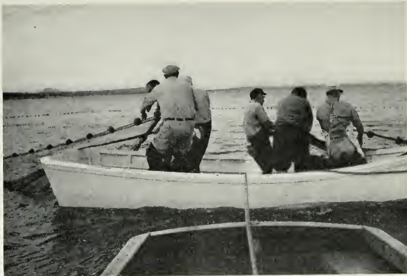
FIG. 27. Sardine fishing in Magdalena Bay, Lower California. The power launch in the foreground keeps the skiff out of the net as the men pull in the wings. The light lampara nets are hauled from the skiff whereas the heavier purse seine is fished from the N. B. Scofield itself. These nets are used for taking sardines in the young fish survey and for tagging as well as for catching tuna bait. Photograph by Merile Stewart.
