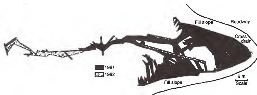
Figure 3 —Map of a typical cross drain sediment deposit over time.
