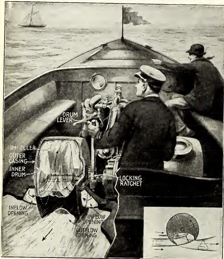
THE WATER-DRIVEN BOAT. INSET SHOWS INFLOWING AND OUTFLOWING STREAMS
