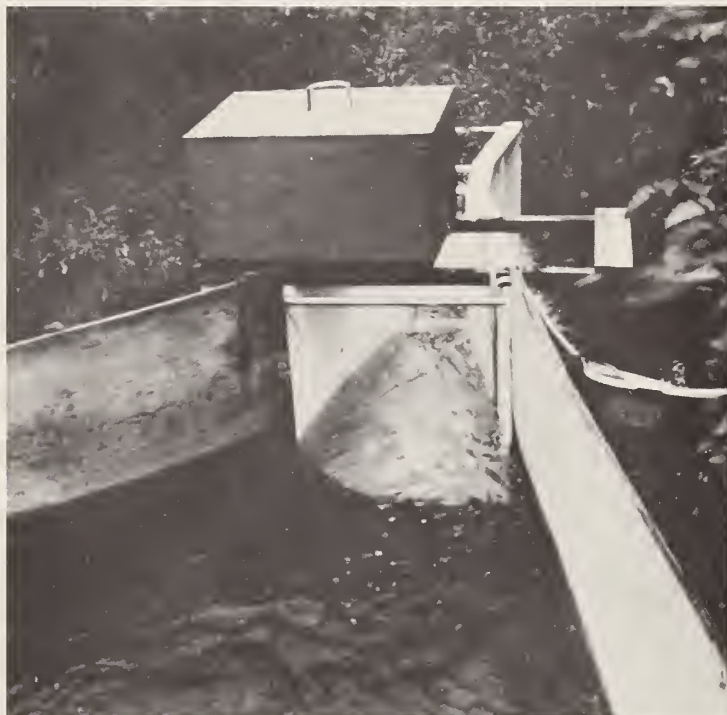
Figure 3.—Parshall flume in C-3 channel, second season after installation. Water-level recorder is in box over stilling well; view is downstream.
