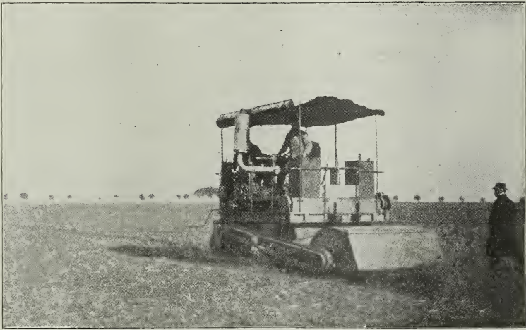
THE KOSZEG IMPLEMENT. Combination Plow and Cultivator.
