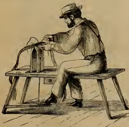
Fig. 2.—BENCH AND CLAMP FOR HARNESS.
