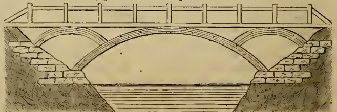
BRIDGE WITH WOODEN ARCHES.
