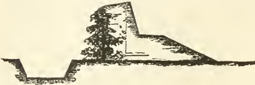
Section of Parapet behind a Hedge and a Ditch in front of it.
