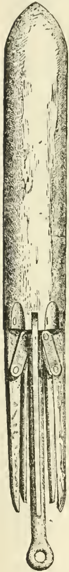
upon the shank being toward the rear, the flukes are kept closed; but, as soon as the projectile reverses,
