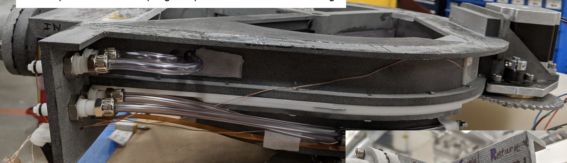
Close up views of air sampling setup in desiccant wheel housing
