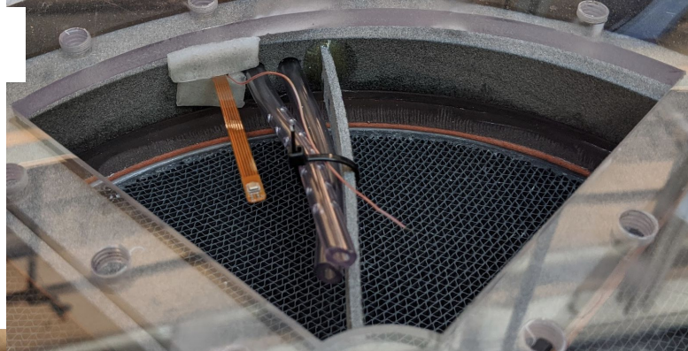
Close up views of air sampling setup in desiccant wheel housing
