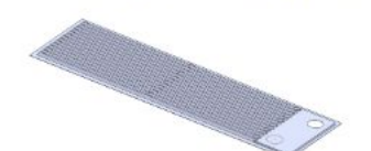
Recuperative HX Core Qt.1 x PolyCarb 1/16" Qt. 2 x ABS 0.060"
