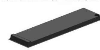
Layer 4 ( Condenser tray ) Qt. 2 x petg .060"
