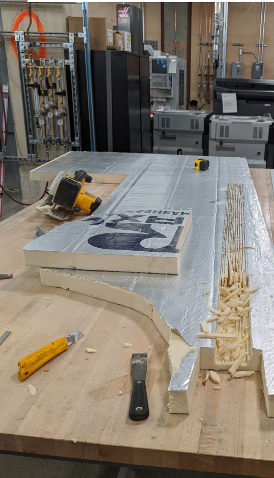
Cutting foam insulation to surround desiccant wheel
