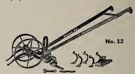
Planet Jr. Double Wheel Hoe No. 12. Equipped with a set of 6 in. hoes, four cultivator teeth, one pair of plows and a set of leaf lifters. The wheels can be raised or lowered and set from 4 to 11 inches apart to fit various requirements. Price \$10.25. Weight 33 lbs
