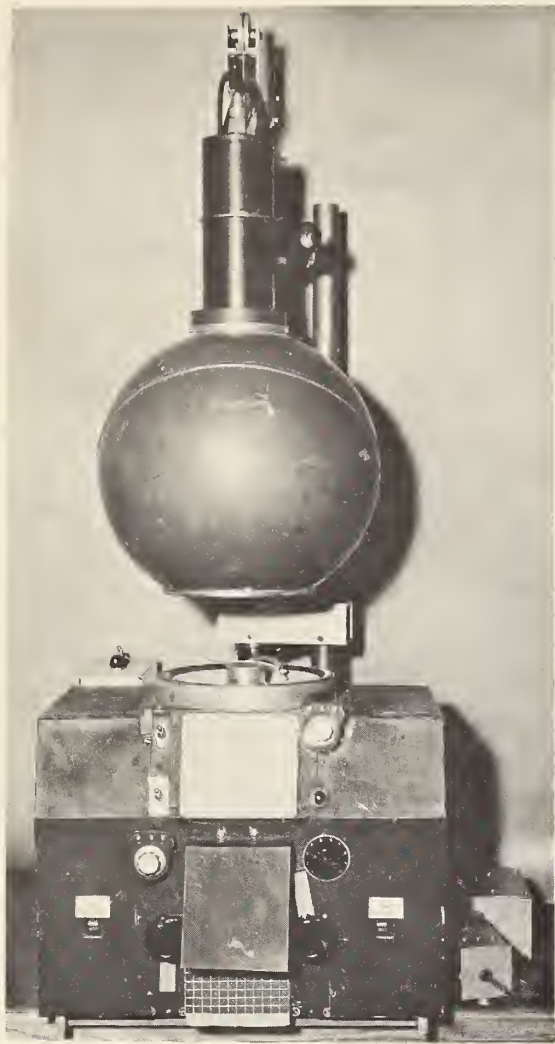
Figure 3.--An assay of phytochrome in the dual-monochromator spectrophotometer starts with centering a sample, such as a bean seedling, so that the 12-inch sphere and projecting phototube can be lowered over it. The oblong base houses the lamp for measuring pigment changes, lenses, mirrors, and other optical parts of the instrument, as well as the electrical measuring equipment. The operator applies irradiation of two pre-selected light waves alternately to the sample, and the meter readings on the dial show the change in phytochrome's form. The amount of change indicates the concentration of the pigment. Wave lengths used have generally been 6600 A. far red and 7350 A. far far red, because these are about the peaks of effectiveness for controlling the plant photoreactions.
