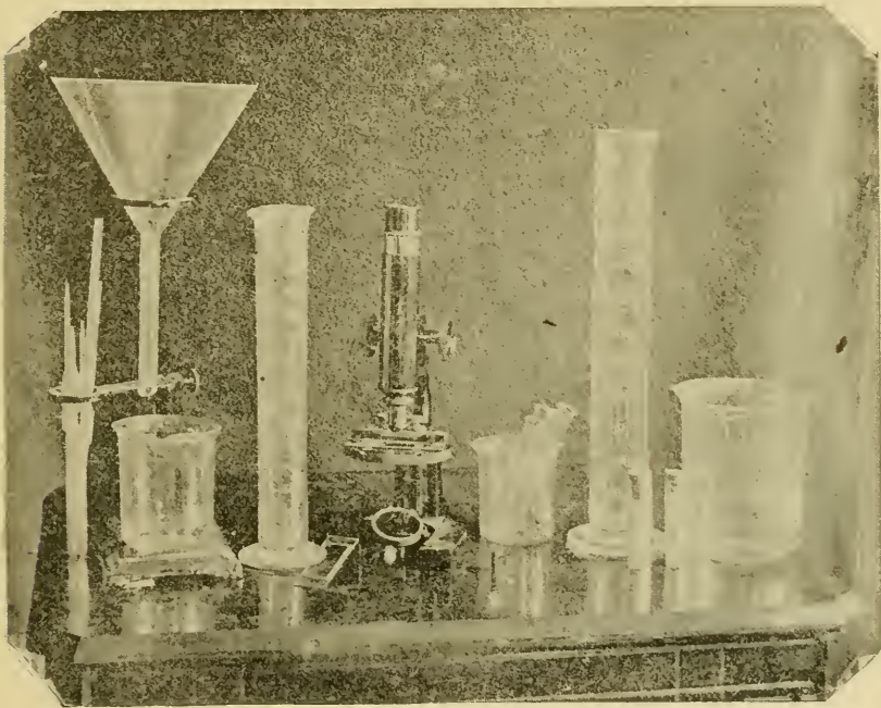
FIG. 3.—COMPLETE APPARATUS FOR BIOLOGICAL EXAMINATION OF WATER.
